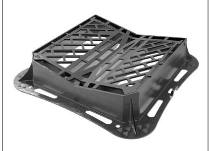
Inspection manhole cover in Spheroidal cast iron EN- GJS-500-7 conforming to norm UNI EN 1563:2004 with load bearing capacity over 400 kN (40 tons), conforming to the load class D400 as set out by norm EN 124-2 2015.
